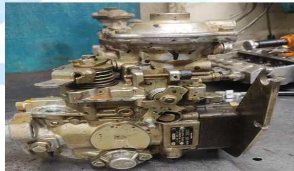
Fig.no.4.4 FUEL INJECTION PUMP
