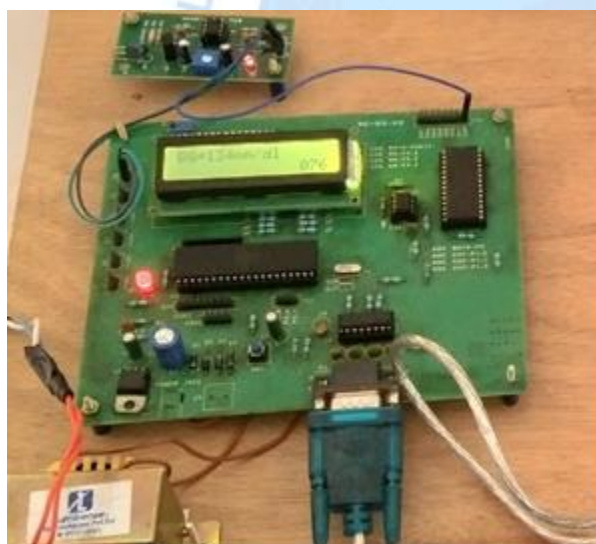
Fig. 8. Final Prototype of A non invasive glucose monitoring device using NIR
