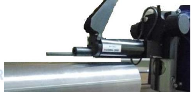
Fig 3.surface roughness measurement setup
