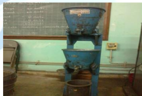
Fig. (4) Slump Cone Test and Compaction factor test
