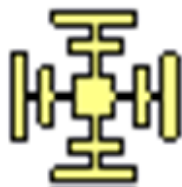
FIGURE 5. The novel SRR structure
